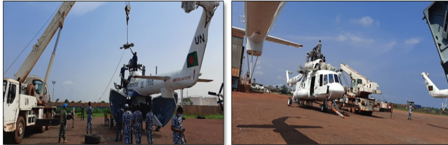
Photo 8: Helicopter Assembly by BANAVN Technicians
